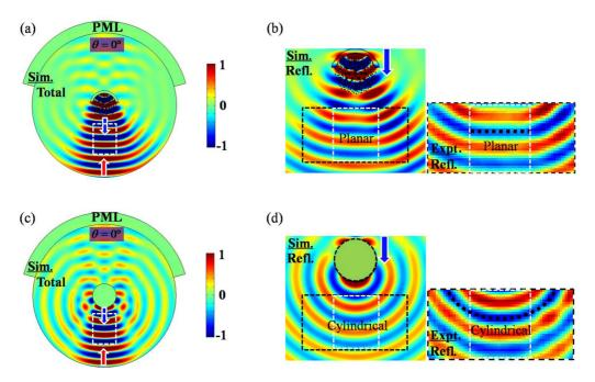
FIG. 3. (a,b) are the simulated total pressure field pattern and the simulated (left) and the measured (right) reflected pressure field patterns from the retroreflector for an incident beam at  $\theta=0^{\circ}$  on the designed retroreflector at 3.0 kHz. (c,d) are the simulated total pressure field pattern and the simulated (left) and the measured (right) reflected pressure field patterns for an incident beam with  $\theta=0^{\circ}$  on a cylinder with  $R_0=0.1$  m.
